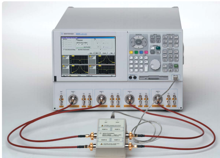
ECal enables fast, accurate, repeatable calibrations 30 times faster than mechanical calibration.
